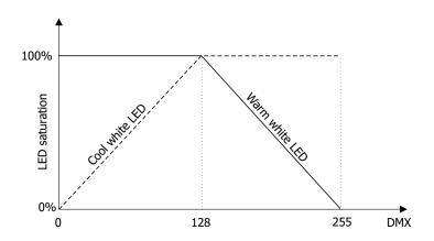
$<sup>^{\</sup>star\star}$  The mode 2 is suitable for control of single colour modules (e.g. ArcLine Optic 12 R,ArcLine Optic 24 G,ArcLine Optic 36 CW, ....)
